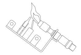
**FIGURE 10. Incorrect Shape of Pilot Flame**
